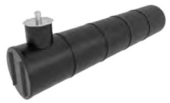
Water reservoir with controls and instruments chamber. Access via dome.
