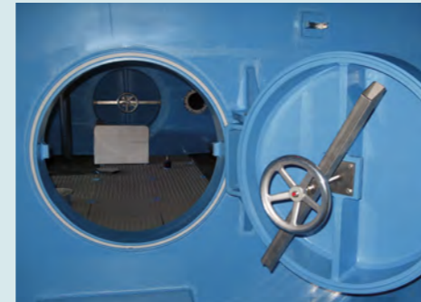
View from the water chamber through the pressurised PE door into the controls and instruments chamber
