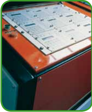
Fig. 37 - Internal pressure creep testing device
