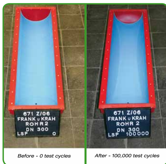
Fig. 60 - PP pipe, DN 300 in abrasion test, FRANK & KRAH Wickelrohr GmbH
