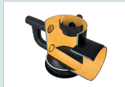
Exterior bypass of a drop structure and overflow to the side
