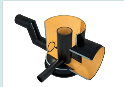
Manhole intake with inside drop/drain pipe
