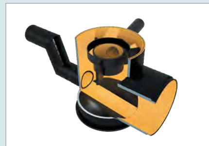
Manhole intake with overflow pot and roughing
