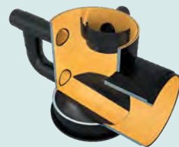
Exterior bypass of a drop structure and overflow to the side
