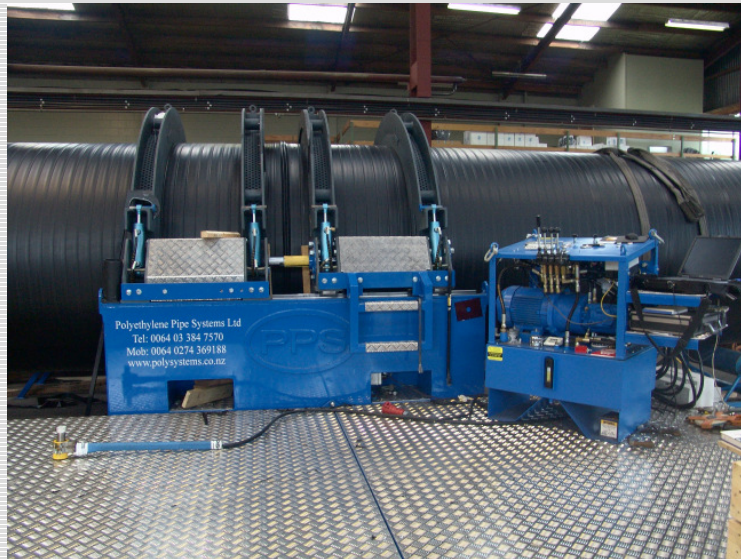
Picture 1: Welding machine for OD 1800mm pipe
