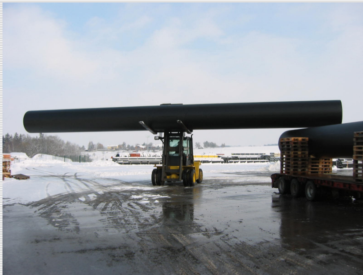
Picture 3: Loading of truck in our factory for transport in Europe (18 m long pipe OD 1400 mm)
