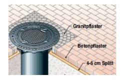
Construction vehicles may only drive over the chamber manifold if it has been designed to withstand traffic loads.
