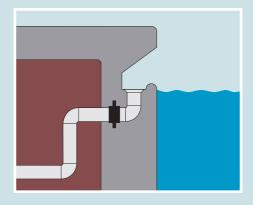
Pre-fabricated wall leadthrough with flange connectors on both sides for easy installation into formwork
