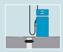
FRANK puddle flange in oil- and gasoline resistant NBR for use at e. g. gas stations.
