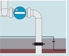
House lead-ins for water supply and discharge pipes as well as for lightning protection earthing strips and ground wire.
