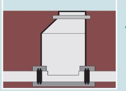
Integration of pipes of any outside diameter into concrete manholes
