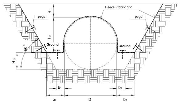
The final mounting dimensions H 1 to 3 and b2 are defined according to the maximum groundwater level and the buoyancy calculation.
