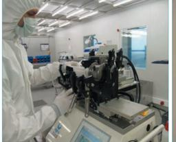
The fully automated welding process and accurate control of the process parameters guarantee short welding times and fast installation of piping systems
