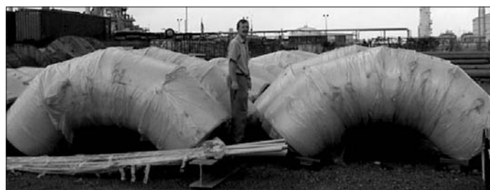
Fig. 3: Segmented bends (PP-H) d1050/SDR 33
